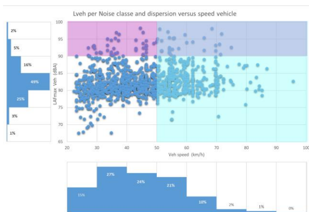
Figure 7. Correlation between vehicle speed and pass-by noise.
