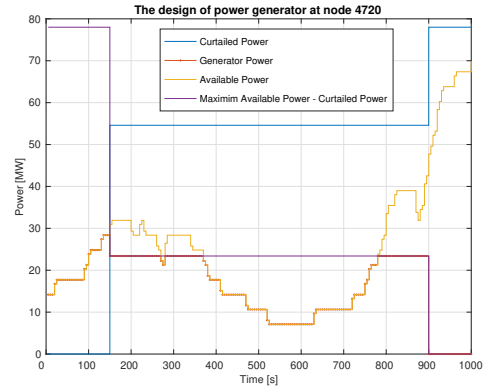
Fig. 2. The power variables in the power generator at node 4720. The P_n^C(k) variable is described by the blue curve, while the violet one depicts \bar{P}_n^G - P_n^C(k) . The yellow line represents P_n^A(k) , and the dotted red one is P_n^G(k) .
