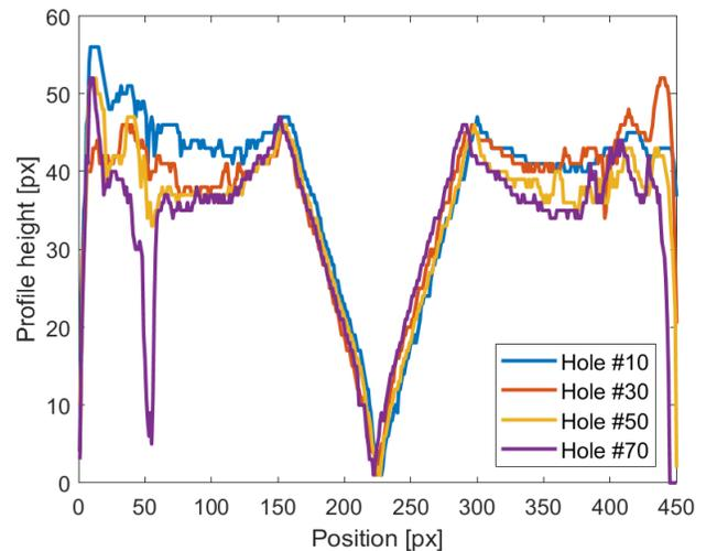
(b) Comparison of drill bit profiles with increasing wear.
