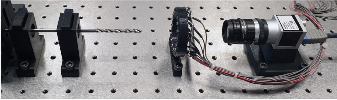
Fig. 2: Realized measurement system on the optical bench. From the left: two drill support, the ring illuminator and the camera on the camera support.
