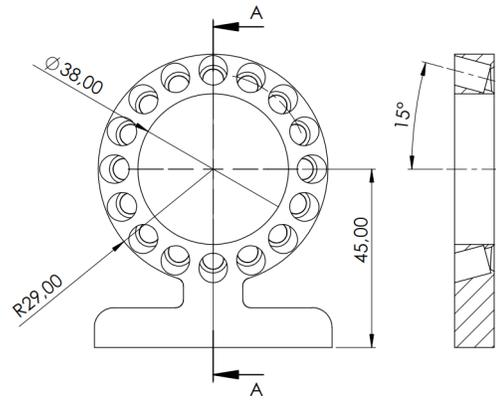
Fig. 1: Dimensional drawing of the custom ring illuminator. All the measures are in mm.
