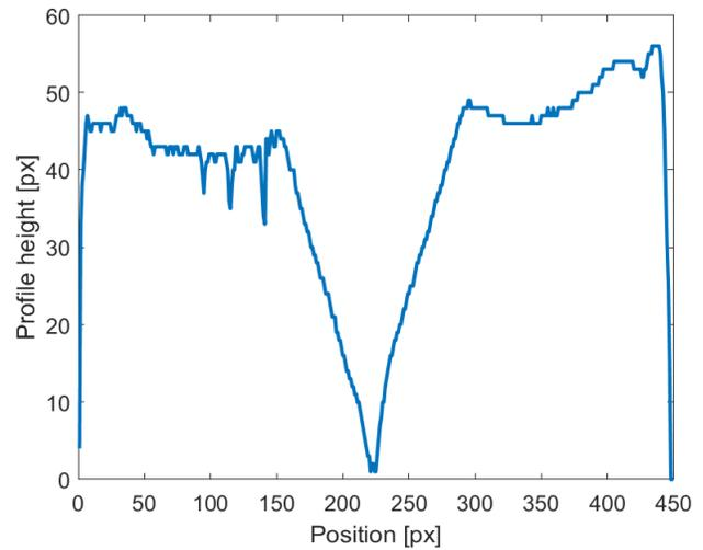
(a) A profile of a new and clean drill bit.
