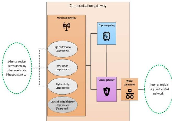
Figure 7: Secure CPS-to-X Connectivity PIARCH [13]
