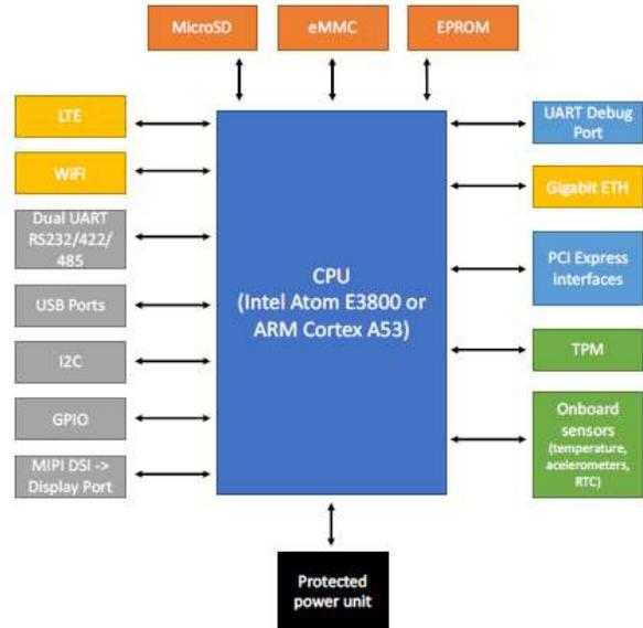
Figure 8: Industrial Edge Computing Gateway PIARCH [16]
