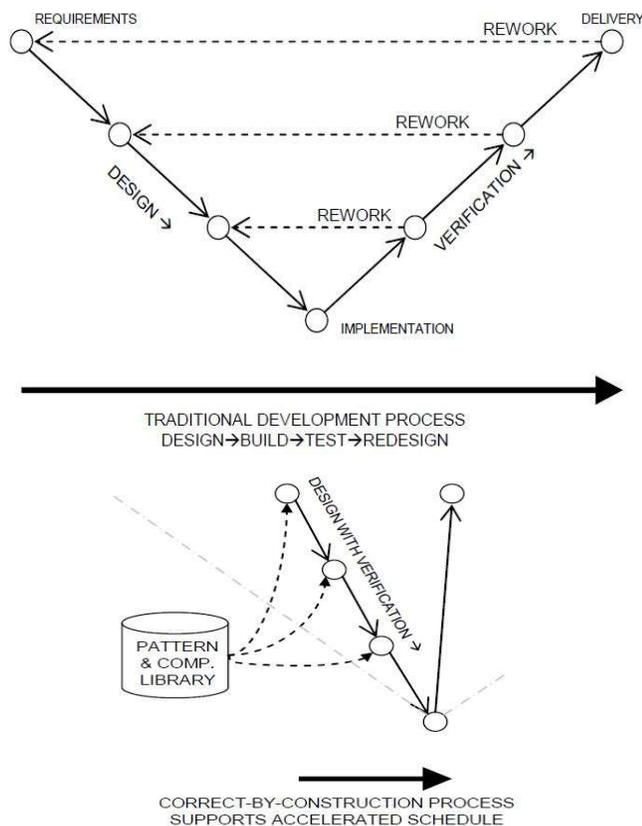
Figure 6: Impact of correct-by-construction development process [10]
