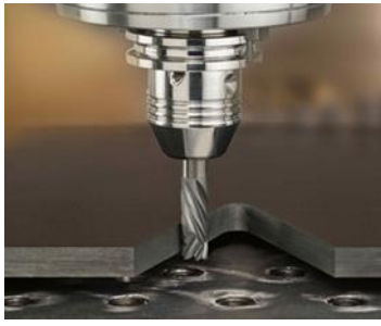
Figure 4 Industrial trimming of a composite part.
