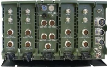
Figure 5 – The Four-channels Software Defined Radio
