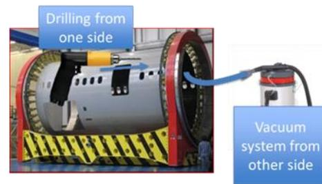
Figure 8 – Automatic Vacuum System
