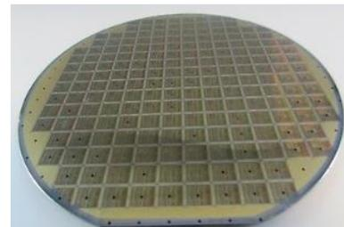
Figure 3 – Example of GaAs wafer produced at the Foundry
