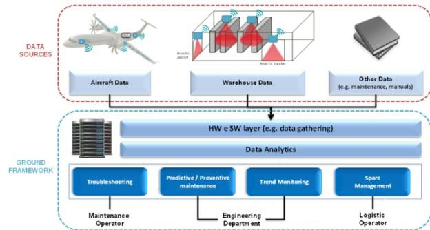
Figure 11 – Overall system description showing both the on-board and on-ground components
