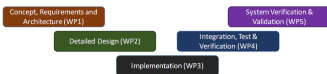
Figure 3 - Math of a V engineering model to the work package structure of cell
