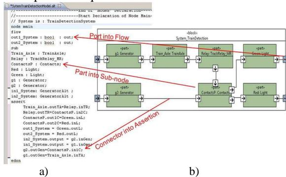
Figure 3: a) Main node declaration in AltaRica; b) Internal block diagram of TDS
