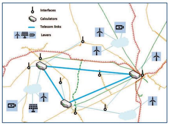
Those area automatons, also called Area Slow Automatons (ASA), are complemented by Substation Slow/Fast Automatons (SSFA) and Centralized Slow Automatons (CSA).
