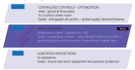
The centralized level handles the global vision and the heavy forecasting computation and provides lower levels with set-points for optimal operation (OPTIMIZE).
