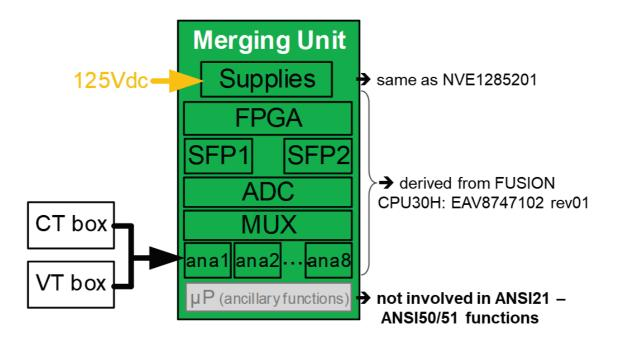
The main idea behind that is to use the simplest possible design to ensure the tasks related to the protection functions, like merging unit, and let the more complex electronics perform elaborated, but less critical functions.
